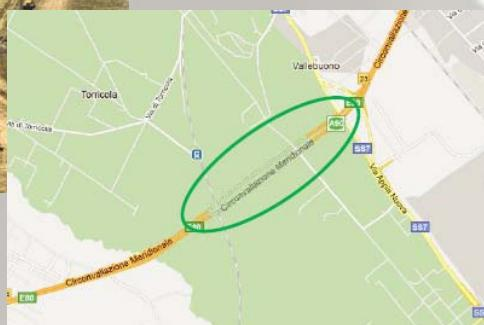
Open to traffic in 2000, it is located along the Rome Ring Road, is a 1150m long tunnel, monodirectional traffic, 3 lanes each 3.75m wide.
