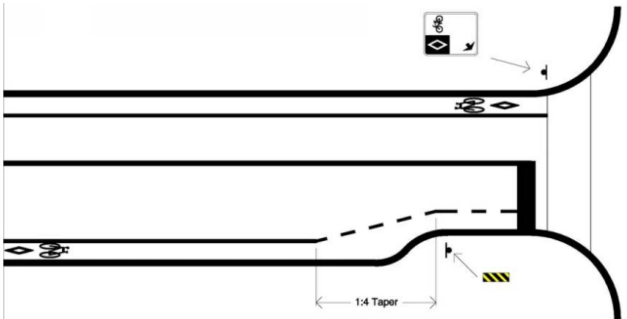
Figure 10: Bike Lane Tapered at Intersection with Curb Extension.<sup>182</sup>
