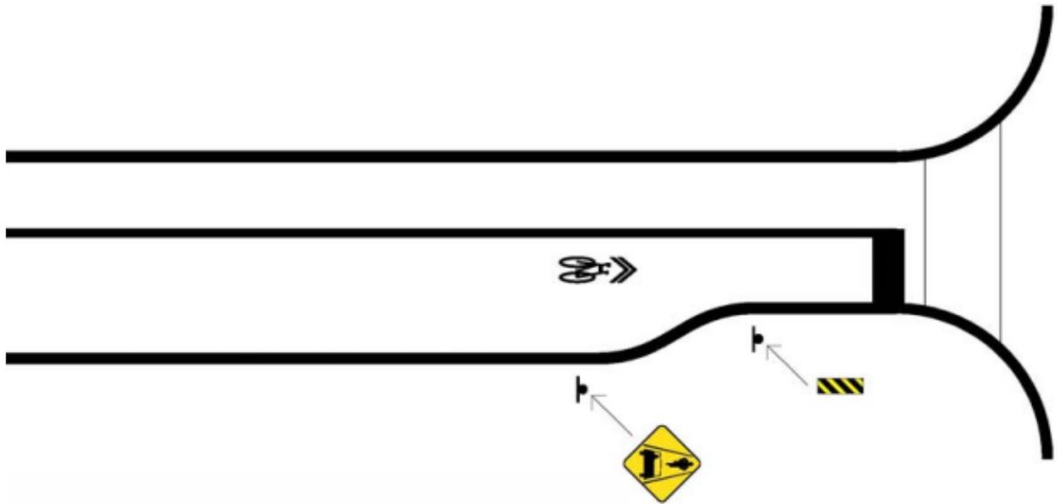
Figure 9: Sharrow Application at Intersection with Curb Extension.<sup>182</sup>
