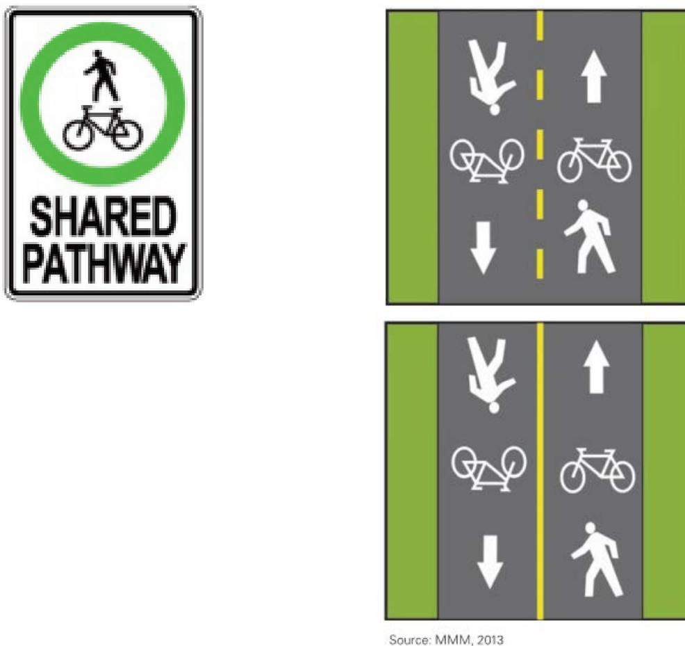
Figure 3: Shared Pathway Signage and Typical Pavement Markings for Shared Use pathway.<sup>180</sup>
