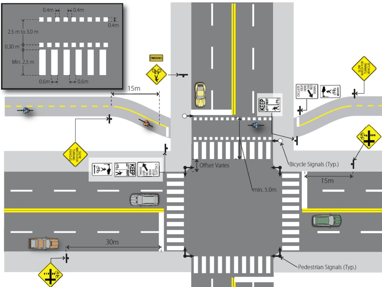
Figure 5: Sample Design Application - Cross-Ride to Facilitate Crossing a Multi-use Trail / Active Transportation Pathway.<sup>180</sup>
