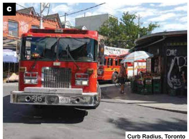
“ Changing the size of the design vehicle used - using a smaller delivery truck instead of a transport, for example - enables the road and intersection dimensions to be narrowed down.”
